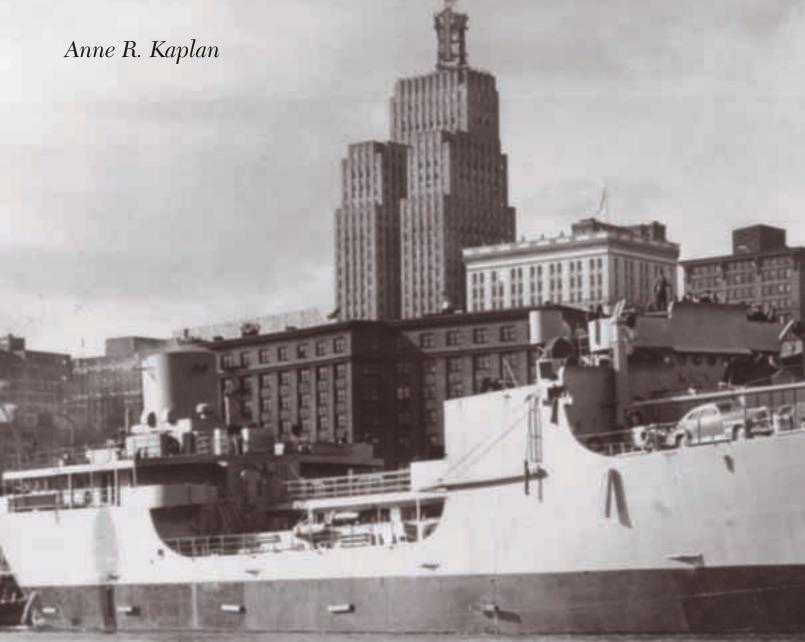
Navy tanker, built on the Minnesota River at Savage, docked in St. Paul on its way to New Orleans, 1944. All parts of the vessel were made in Minnesota, including the guns by Northern Pump of Fridley. The vessel was 325 feet long and 55 feet high; it drew 9 feet empty (18 feet when loaded).
