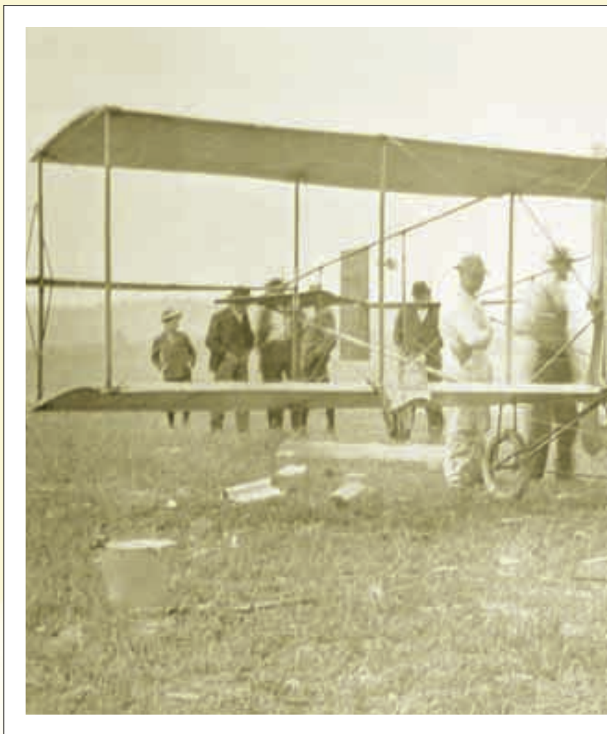
Grounded for repairs, September 1911; note broken metal struts, extra-capacity gas tank (behind the radiator), and pails used to bring water to the radiator.
