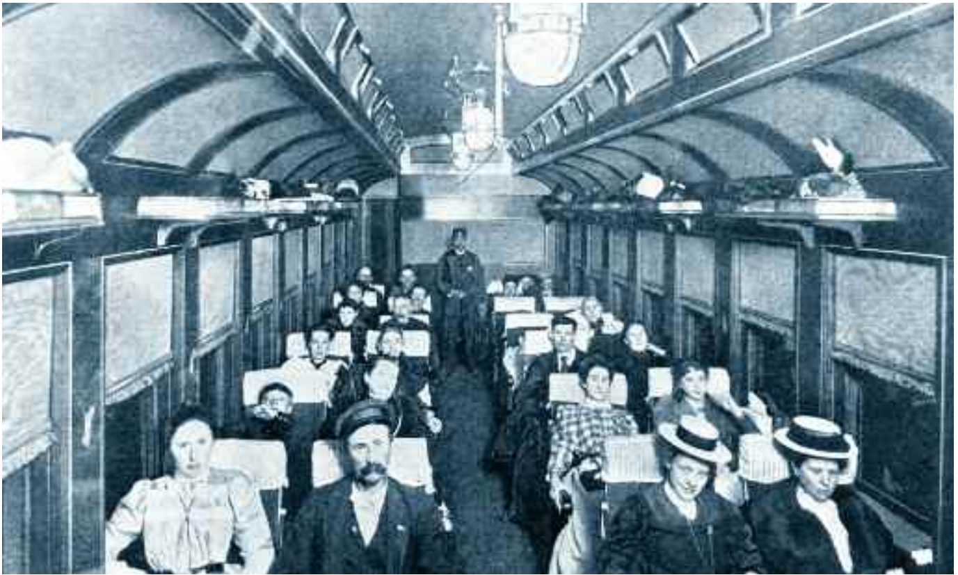
By 1900 passenger cars on Minnesota rails such as this one photographed by “flash light” at 8 P.M. on the Great Western Limited to Chicago featured individual reclining chairs, gas lighting, and steam heat.
