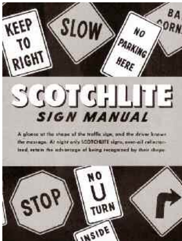
Promotional material, 1945, for Scotchlite ™ , a light-reflective coating made of glass beads and used for highway markings, signs, and clothing. The product was first field-tested on a Minneapolis traffic sign in 1939.
