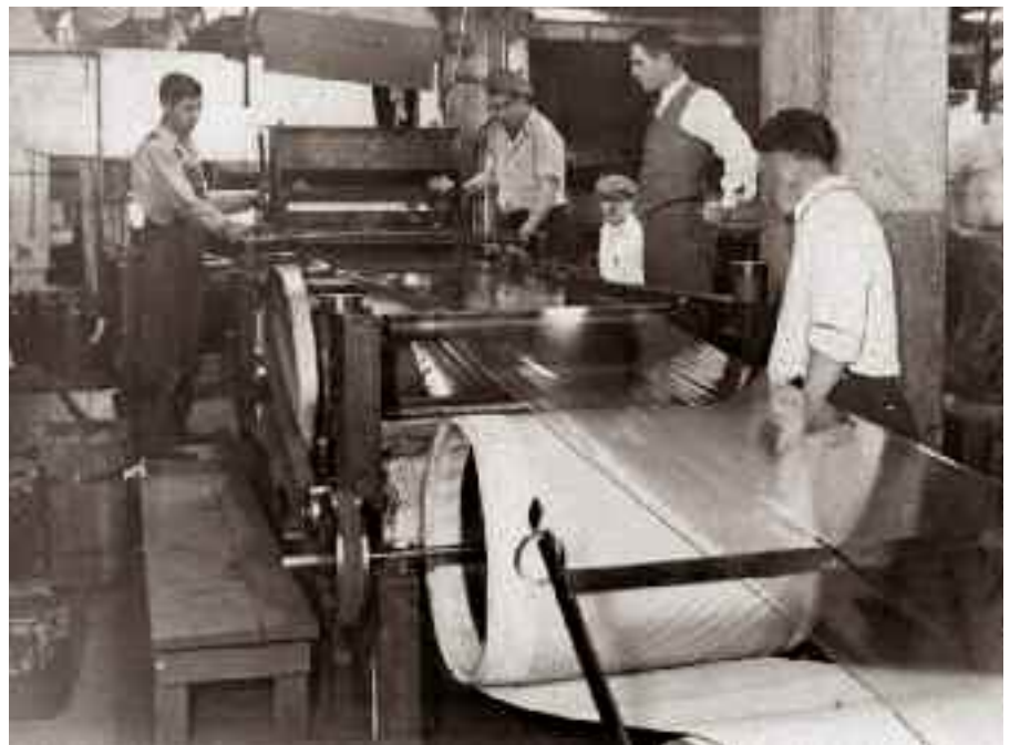
Manufacturing Scotch® Tape at 3M's main plant, St. Paul, 1931. The original tape was adhesive on cellulose, but 3M soon switched to cellophane (developed by the DuPont Company in 1927), and Scotch® Tape began to resemble the product we know today.
