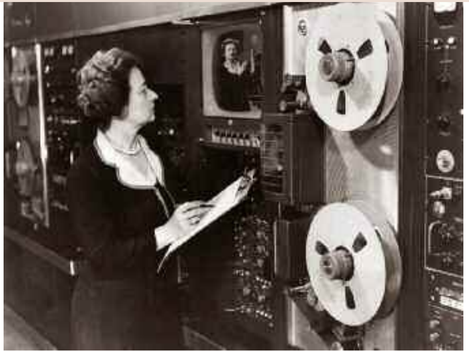
Playback of video recording, 1963. Developed from magnetic audiotape, 3M's video-tape first recorded television broadcasts in 1954.
