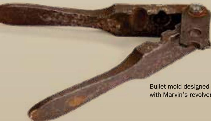
Bullet mold designed for use with Marvin's revolver
