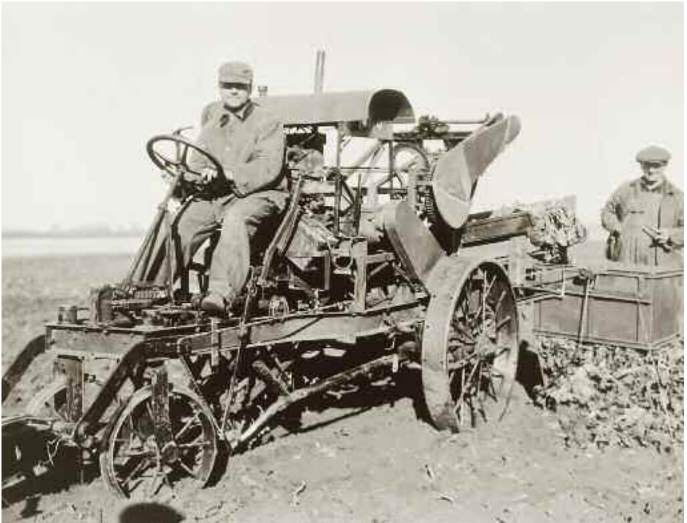
Machines such as this Rassman beet lifter and buncher, tried in the Valley in the 1930s, offered hope of reducing the number of hired workers.
